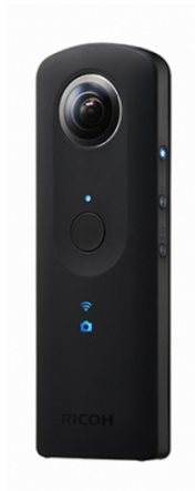
Figure 3.1: The Ricoh Theta S camera. It contains two cameras, one on each side, having field of view of about 220^\circ each, allowing sufficient overlapping space between the two images in order to achieve better stitching, and as a result less distorted 360^\circ panoramic images.
